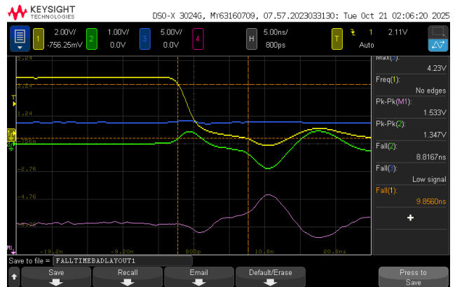
Figure 15: falling edge for bad layout
